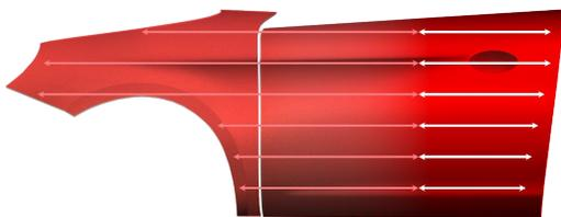
Apply the first coat of the tinted Clearcoat to the repair part and extend into the adjacent panel. Ensure you cover the fade-out zone of the Basecoat.
