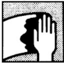
Abrade the surface with a coarse sanding disc removing all loose and flaking rust/paint. Dust off with an air gun. Wipe clean surrounding areas with RALI Wax & Grease Remover (refer data sheet).
